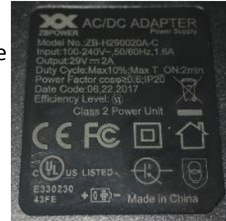
Transformer: Plugs into wall outlet
